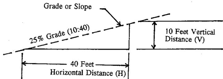
$$\text{SLOPE CALCULATION} = V / H$$
